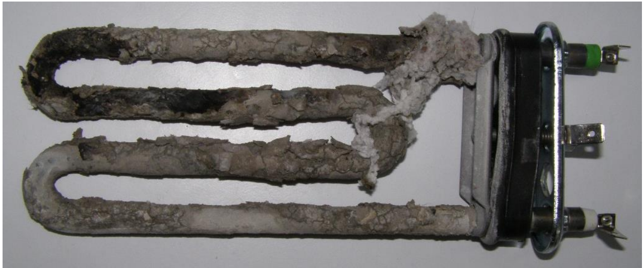
Figure 3.21. Contaminated and calcified heater
