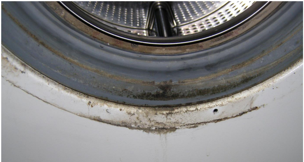
Figure 3.22. Worn-out door seal
