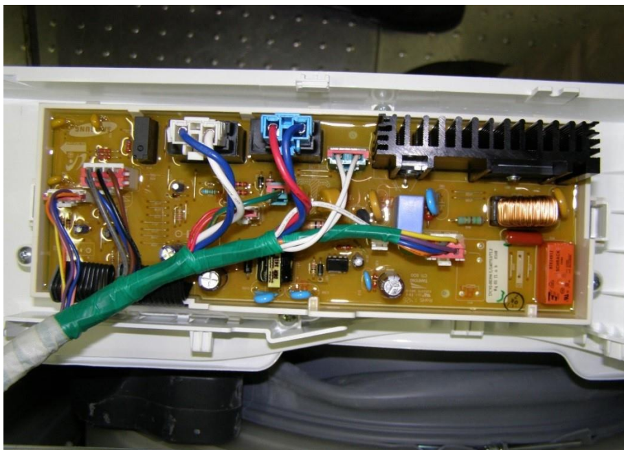
Figure 3.42. Resin layer electronic — technicians generally replace the whole board, but repair or substitution of components on the printed circuit board are possible. However, this type of layer cannot be re-soldered and components cannot be replaced, in case of failure it
