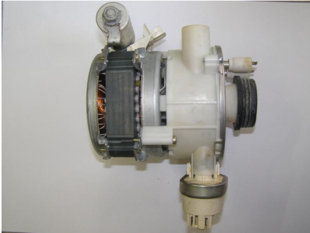
Figure 3.41. Circulation pump without electronic board — seals, pump, heater and motor are separable and their replacement does not require the whole unit to be replaced
