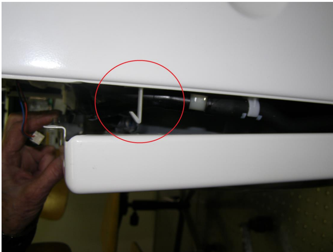
Figure 3.24. Plastic snap-fit used as a connector for the housing of a washing machine (front) — fragile connectors can easily be broken by technicians during repairs or maintenance
