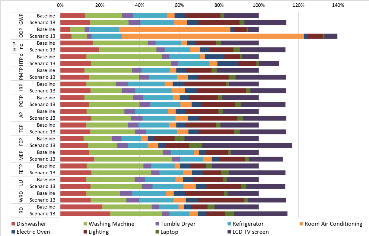
Figure 45. Scenario 13 in comparison with the baseline scenario (with total from the baseline set as 100%) – split into the contributions of the various product groups. (For the abbreviations see table note of Table 42)
